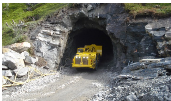
Figure 2.5. Low height mucking and transport equipment (Photo: Werner Stefanussen).
