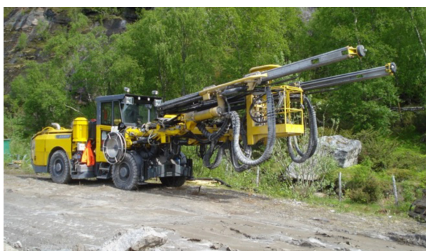
Figure 2.4. Small size 2-boom tunnel machines (Photo: Werner Stefanussen).
