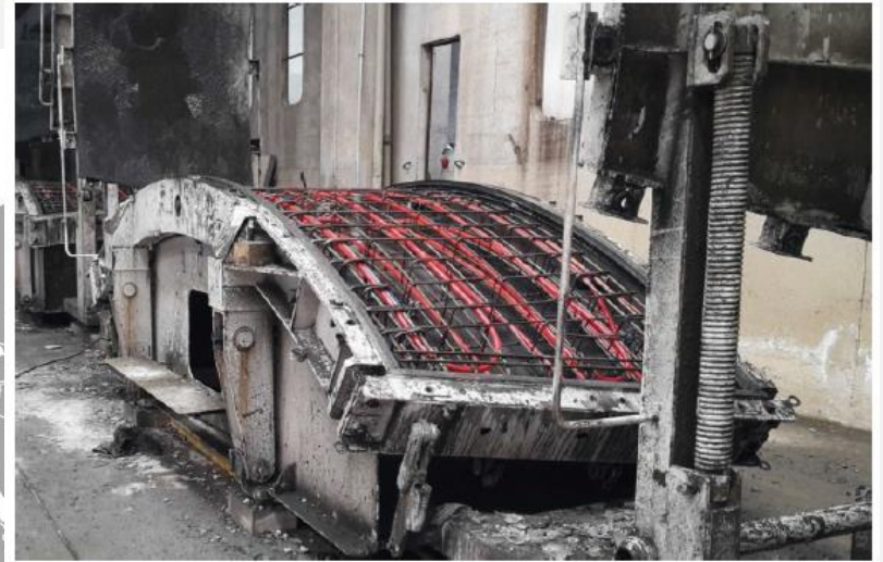
Fig. 4 A thermally activated tunnel lining segment with embedded absorber pipes during its construction (modified from [4]).
