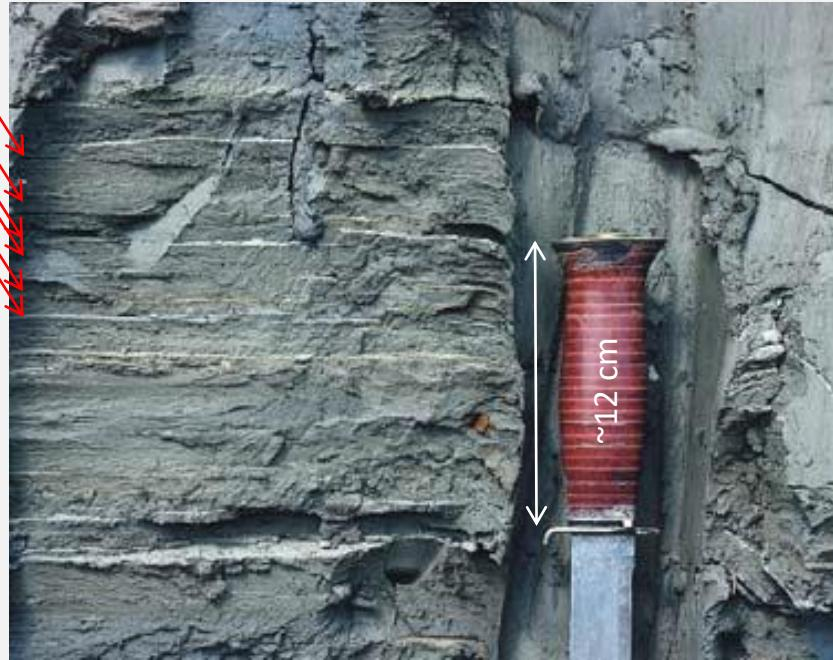
1-2cm clay layers? Silt, fine sand 1-3 mm?
