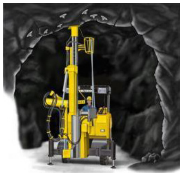
Figur 4.1 Fullmekanisert bolterigg 4.1.3. Tunnelborerigg
