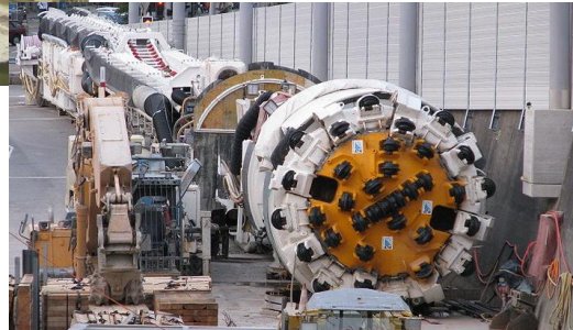
Gripper TBM Escape tunnel
