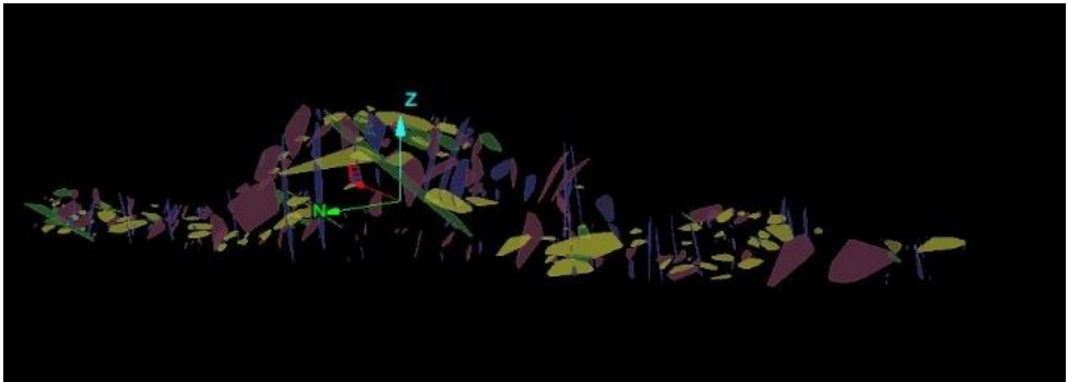
Fig 9 B. Digitally mapped discontinuity sets on the same slope profile as Fig 9A.
