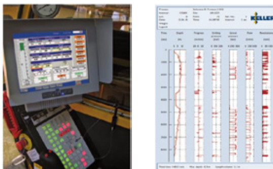
Fig.4: Soilcrete® Process Monitoring, left: live-time process parameters in machine, right: typical process data sheet for each single element executed
