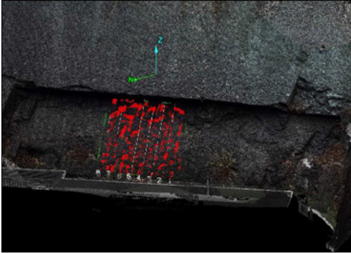
Fig 7A. An example of an area of a rock surface selected for a waviness query. In this example, eight profiles spaced 1m are analysed to determine the maximum asperity amplitude per profile.
