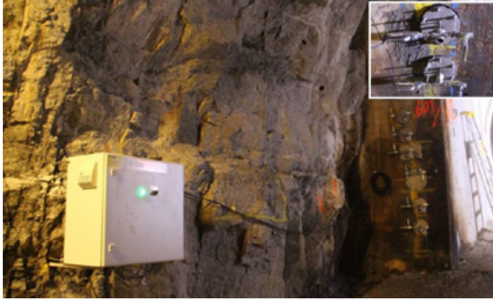
Figure 6. Arrangement of pressure transducers and datalogger. Arrangement of sensors and deaeration valve is shown in top right corner.
