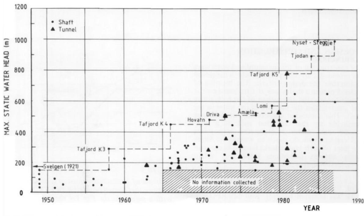
Fig. 10.1 Development of Norwegian unlined high pressure tunnel and shafts
