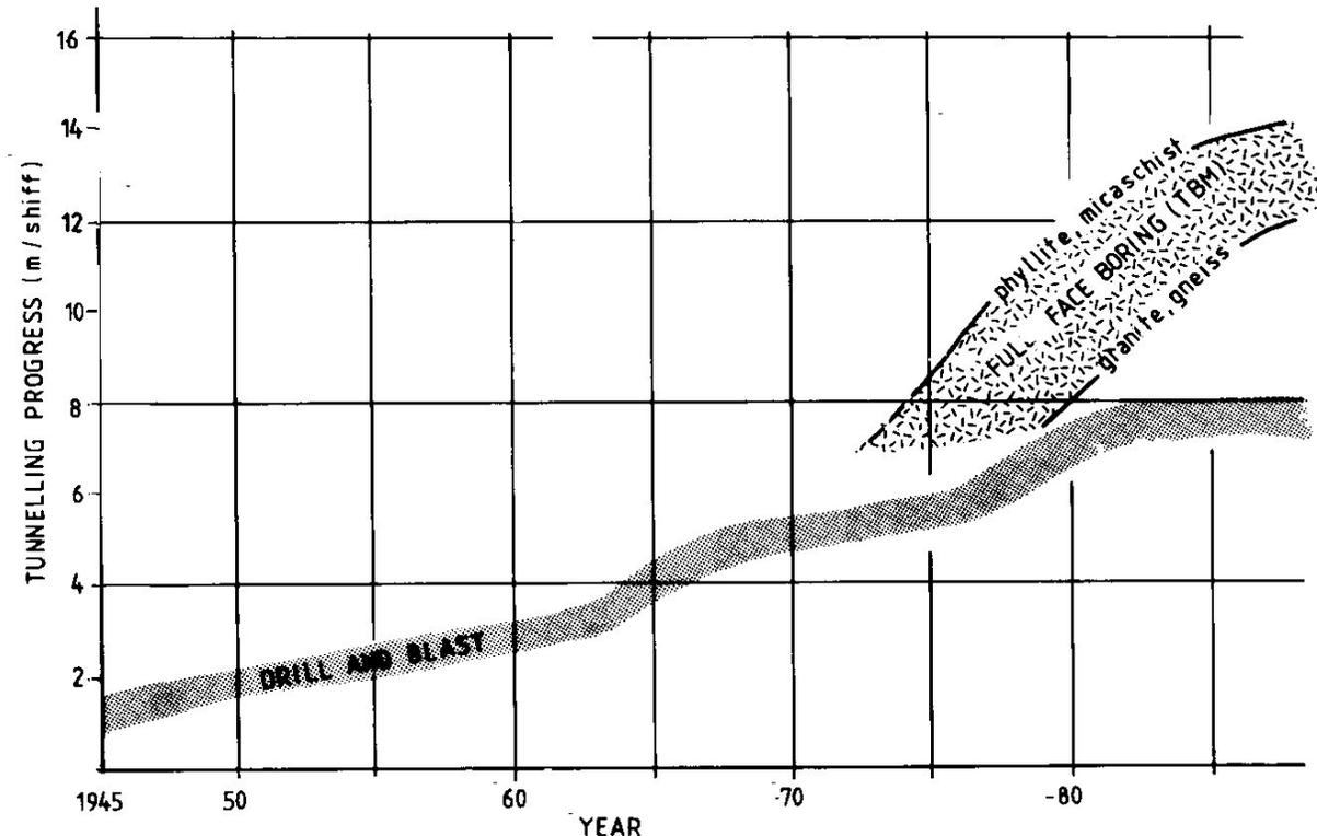
Fig. 1. Development in Norwegian hard rock tunnelling progress (rock supporting works excluded)
