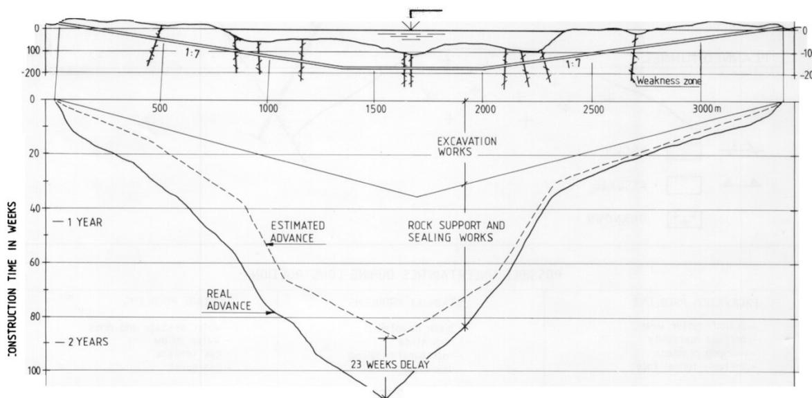
Fig. 9.3 Advance diagrams. Sub sea tunnel driven from both sides
