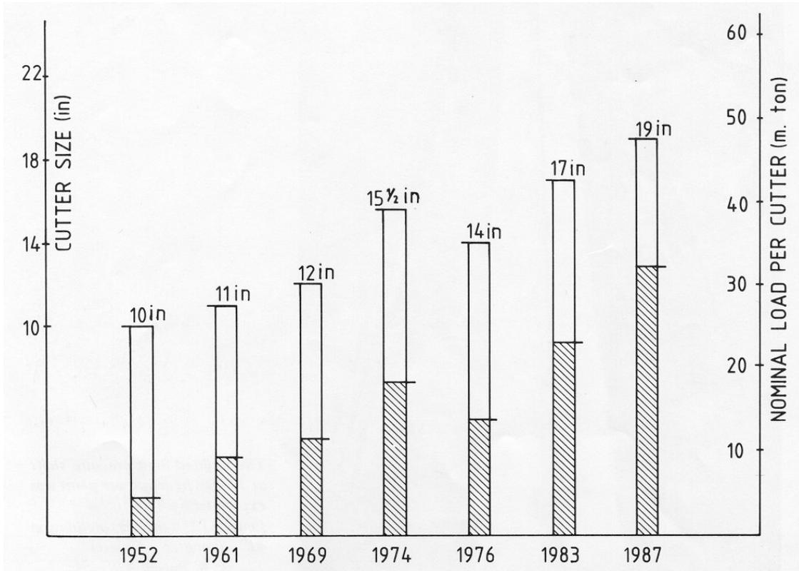
Fig. 18.3 Development towards larger disc cutter size and cutter head
