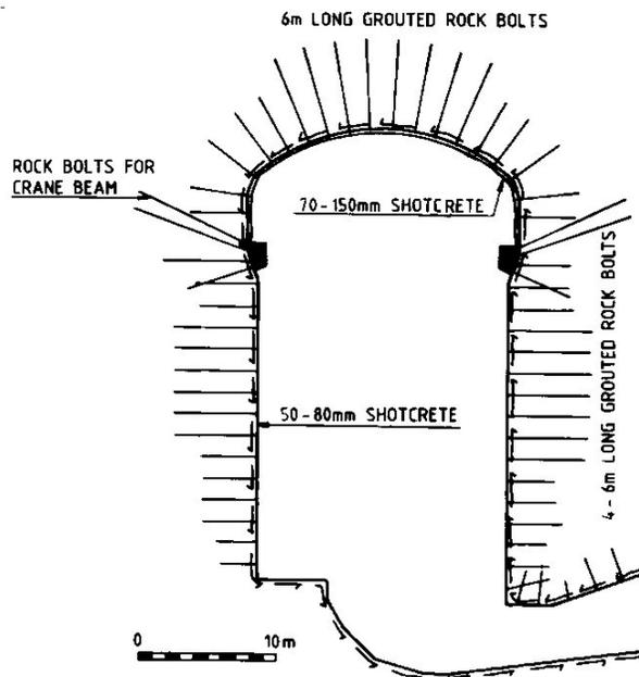
*Fig. 12.1 Modern rock support of cavern roof and walls, and rock bolted crane girders*
