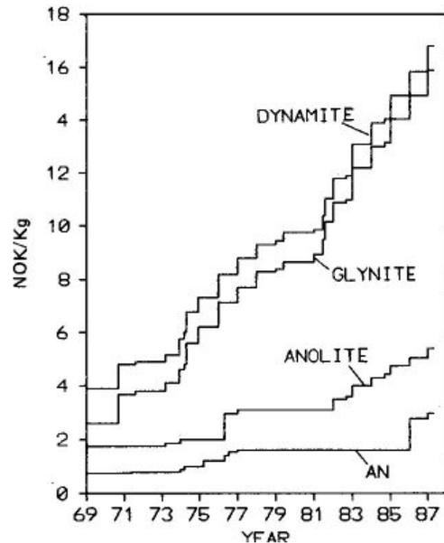
Fig. 2.6 The price gap between cartridge-NG-explosives (dynamite, glynite) and bulk ANFO is still widening (Prices in NOK, 1987 exchange rate: \$1 = 6,80 NOK)
