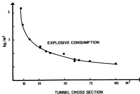
Fig. 2.3 The basic explosive for Norwegian tunnelling today is ANFO. The explosive consumption per m<sup>3</sup> of rock varies widely dependent on cross-sectional size and rock quality
