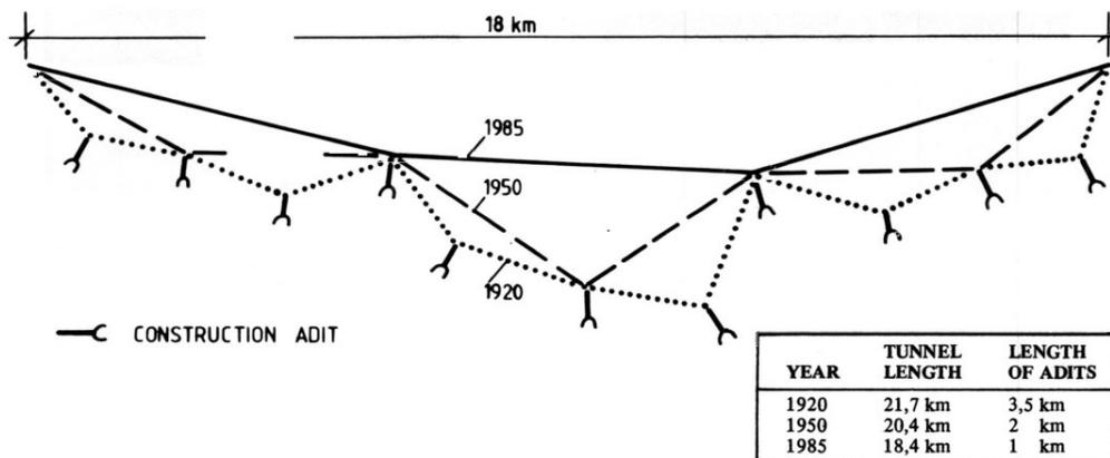
Fig. 1.6 Different tunnel alignments for a tunnel between the two reservoirs "A" and "B". The construction time is 21/2 years in all cases
