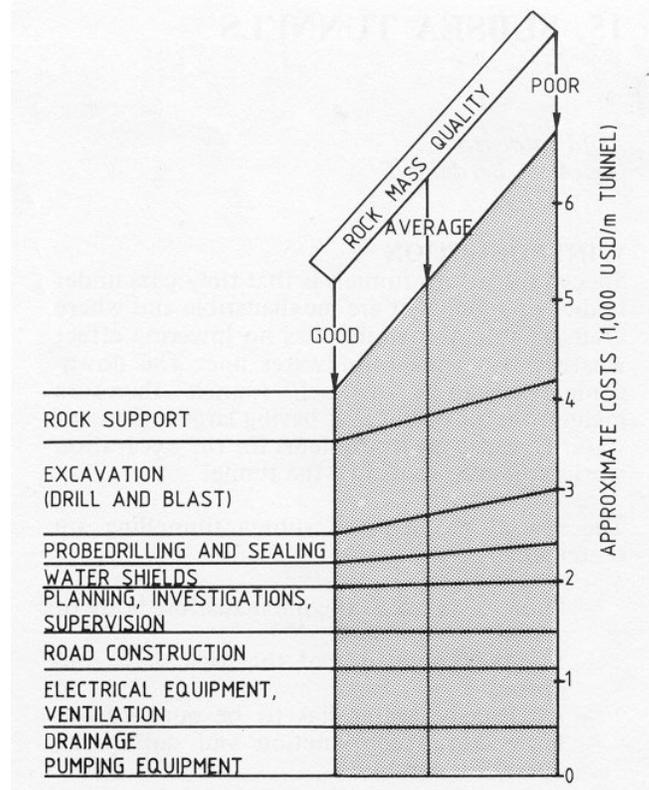
Fig. 15.3 Breakdown of costs for a two-lane sub sea road tunnel
