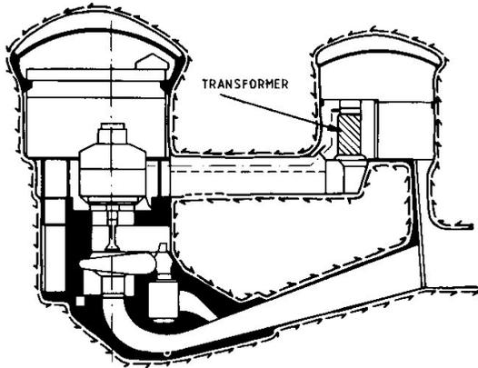
*Fig. 12.3 Transformers in cavern with draft tube gate hoists*
