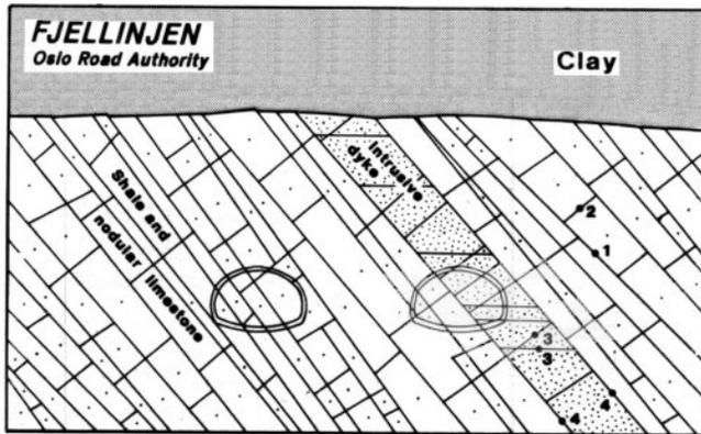
Fig. 8.3 Assumed rock geometry for discontinue modelling of the Fjellinjen road tunnel.
