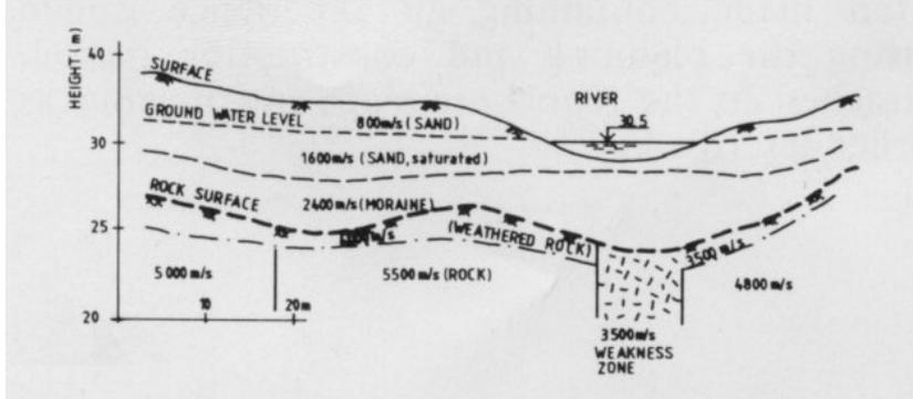
Fig. 6.1 Refraction seismic measurements are often used for rock mass quality evaluation and to find depth of loose materials.
