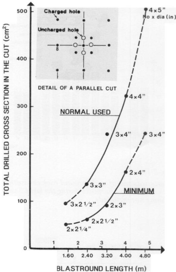
*Fig. 2.4 The length of the blast round depends on rock quality and on the volume of the unloaded opening holes in the parallel cut*
