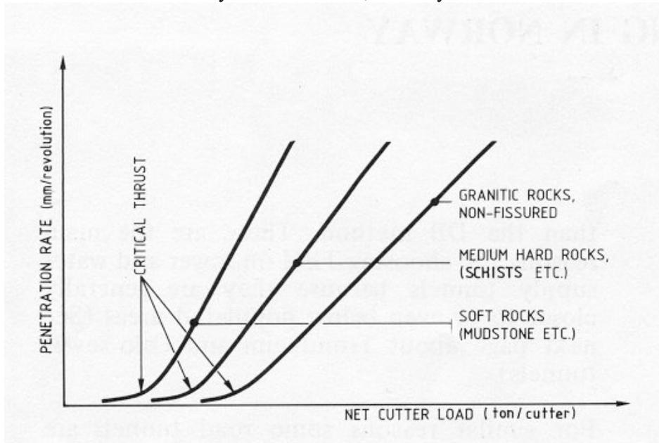
Fig. 18.1 Relation between cutter head and penetration rate
