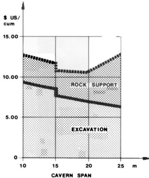
Fig. 13.2 Cavern cost as function of span width
