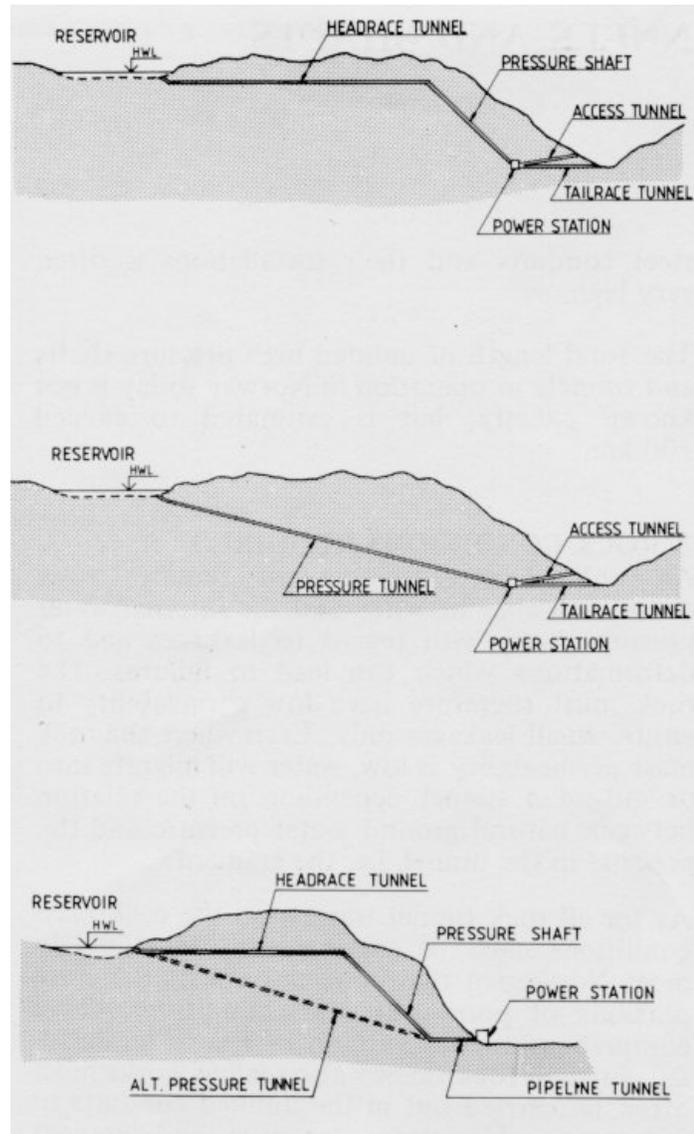
*Fig. 10.2 Different design solutions with unlined pressure tunnels and shafts*
