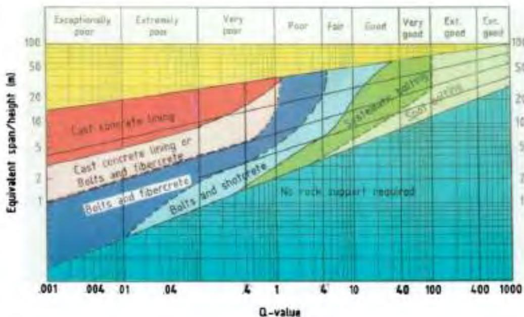
Fig. 8.1 Simplified diagram for design of rock support based on the Q-system
