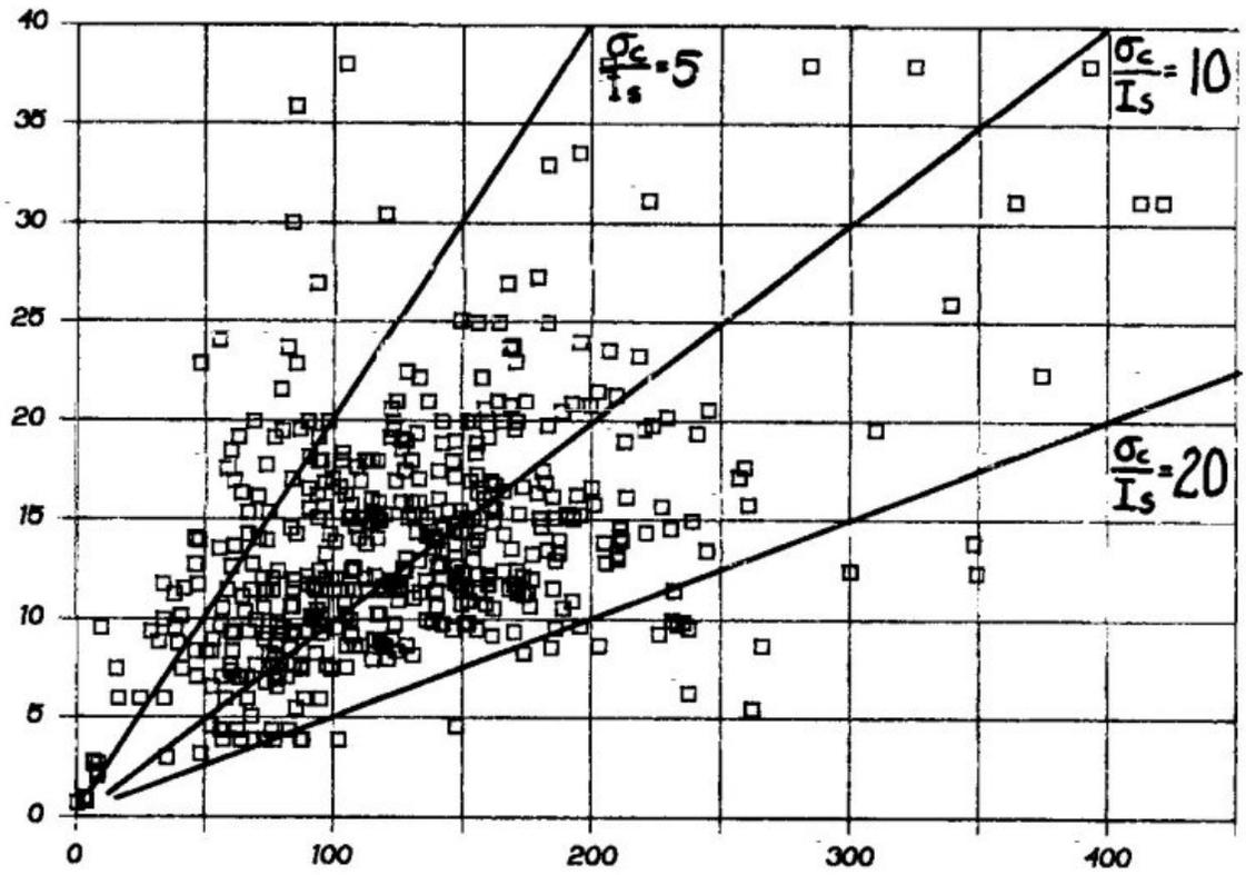
Fig. 4.2 Tensile strength vs. compressive strength.
