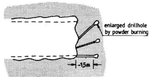
Fig. 1.3 Only 9 holes were used to blast the 12 m<sup>2</sup> tunnel at Follafoss power plant in 1919
