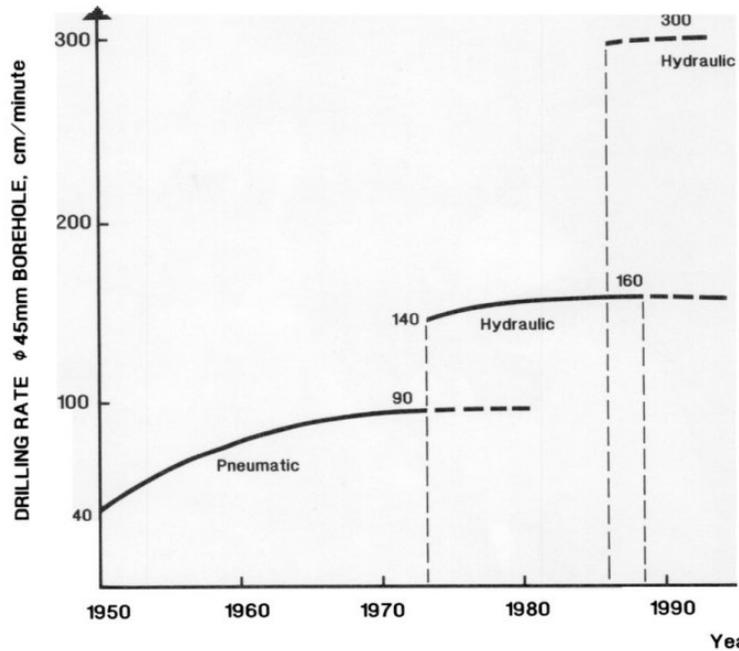
Fig. 2.5 Blast hole drilling rates have been greatly improved during the last decades
