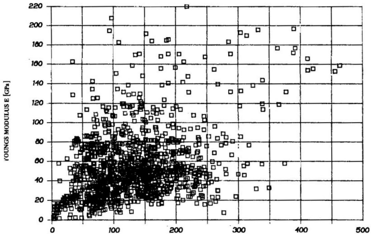
Fig. 4.1 Modulus of elasticity vs. compressive strength.
