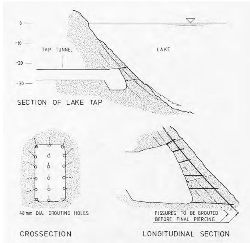
*Fig. 17.2 Leakage cut-off before lake tap piercing*
