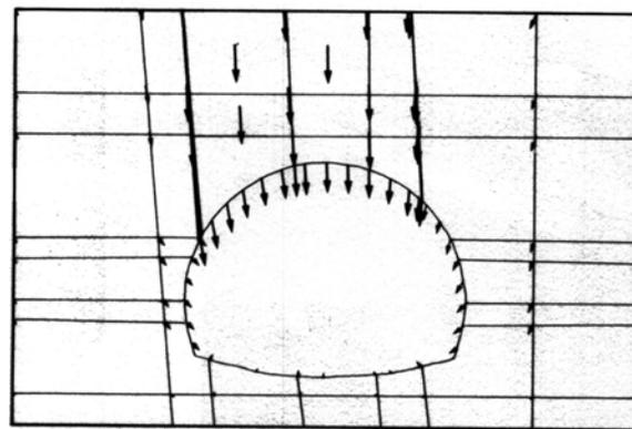
*Fig. 8.2 Discontinuum modelling of tunnel stability problems in jointed rock. Arrows show deformation vectors ( max. 9.7 mm) and line thickness shows shear magnitudes ( max. 6.7 mm)*
