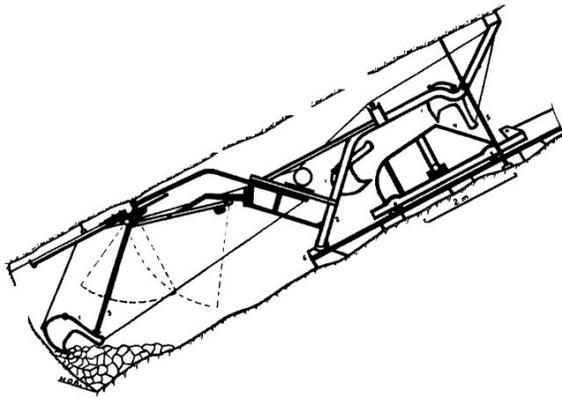
Fig. 1.7 The Larsen shaft sinking rig could be used at angles up to 42°
