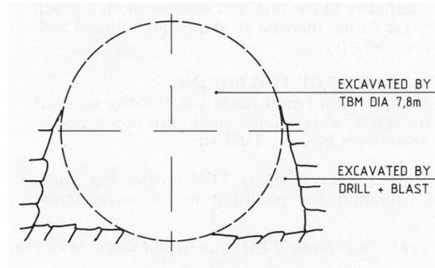
Fig. 18.2 TBM bored road tunnel in Bergen
