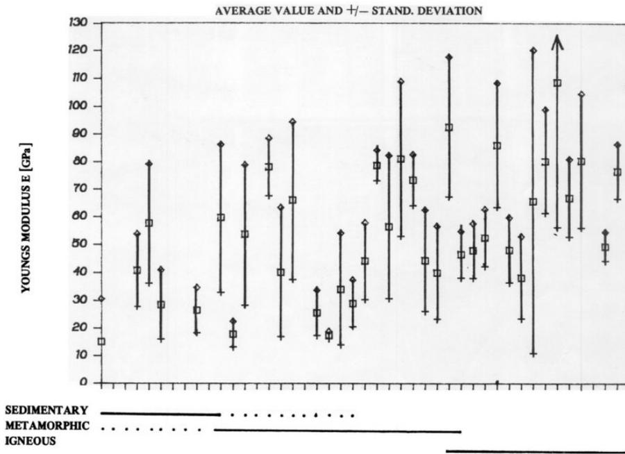
*Fig. 4.4 Modulus of elasticity for various rock types*
