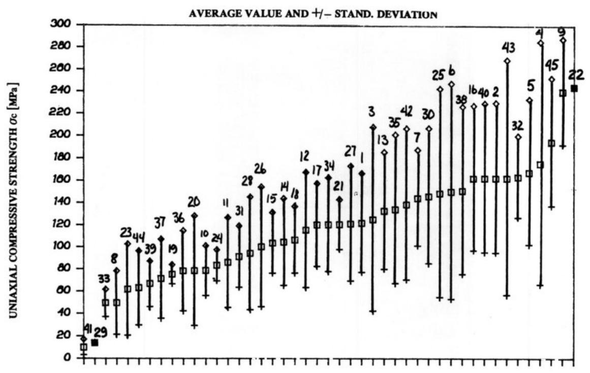
Fig. 4.3 Compressive strength for various rock types.
