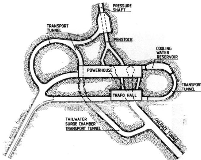
*Fig. 12.4 Example of layout for an underground power station*
