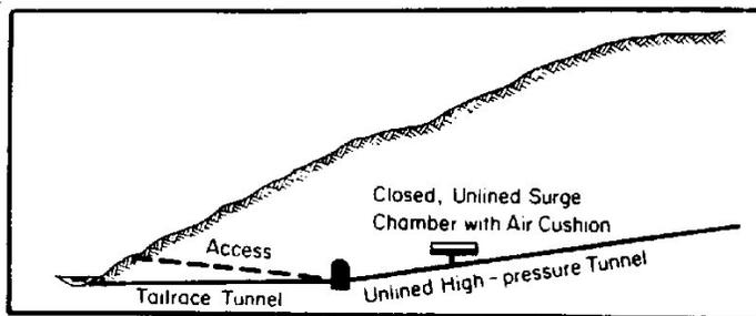
Fig. 11.2 Air surge chamber located at the end of the headrace pressure tunnel
