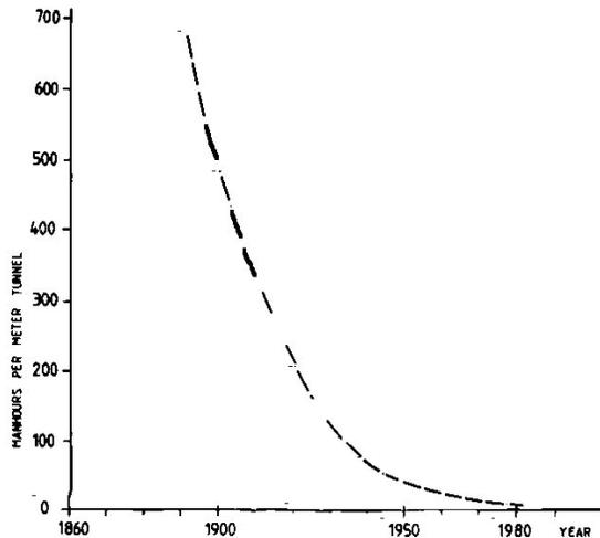
Fig. 1.2 Time consumption in tunnel excavation
