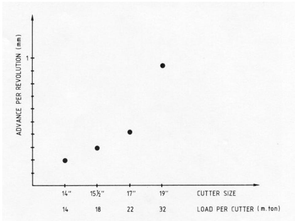
Fig. 18.4 Advance per revolution in relation to cutter size in granitic gneiss (Advance with 19 inches cutter is assumed based on experience with other cutters)
