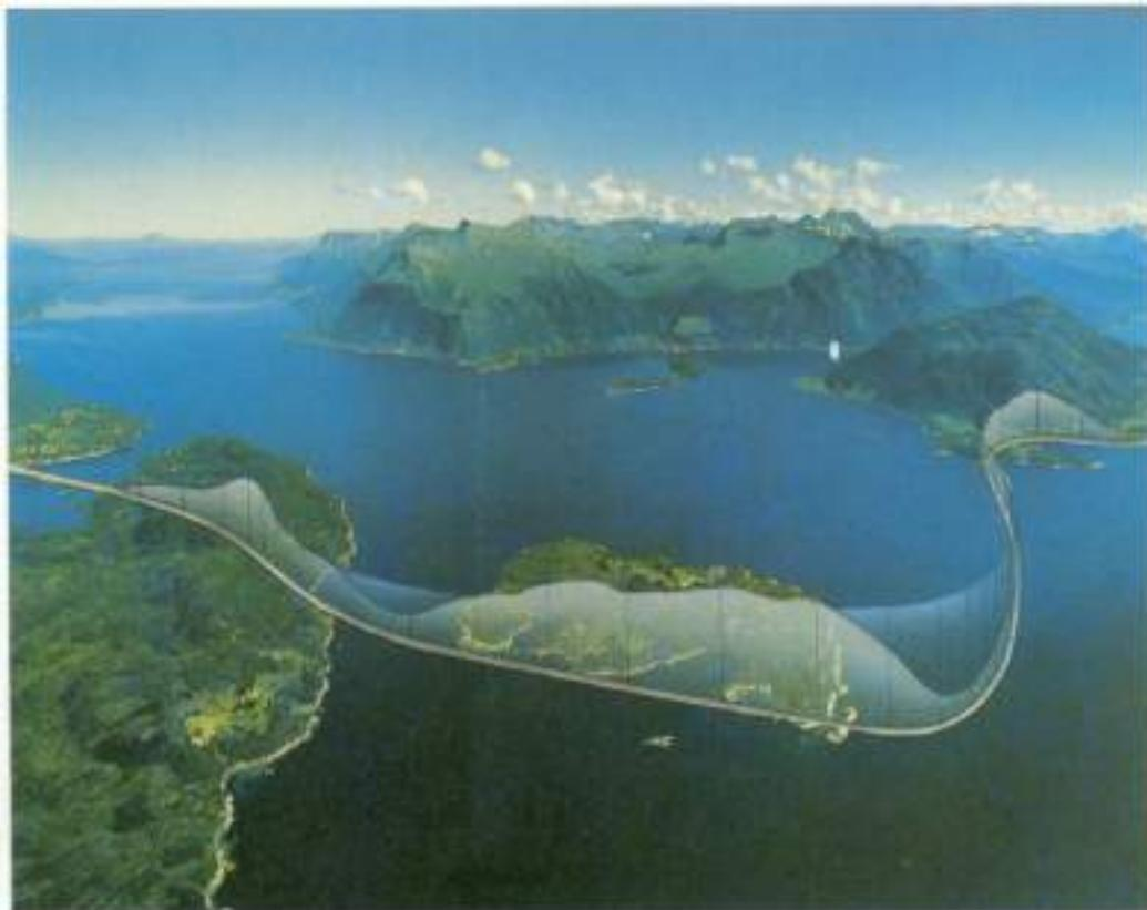
*Fig. IV The planned Eiksund fjord tunnel will improve communication to a large island. Sub sea tunnelling is a Norwegian speciality (Eiksundsambandet)*
