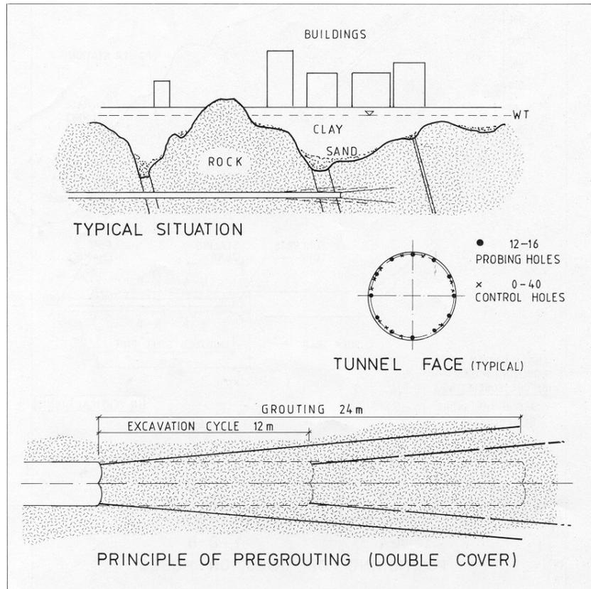
Fig. 17.3 Principles of probing and pregrouting to ensure minimum water leakage into the tunnel
