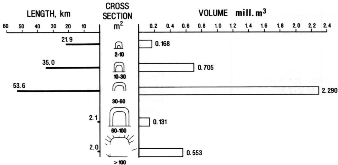
Fig. 2.2 Length and volume of various size tunnels excavated during the year 1985
