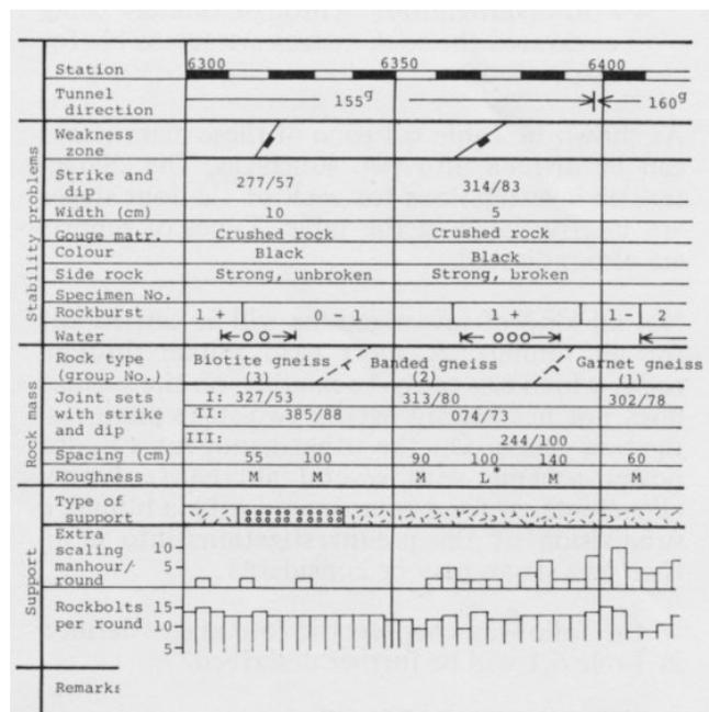
Fig. 6.3 Examples from tunnel mapping.
