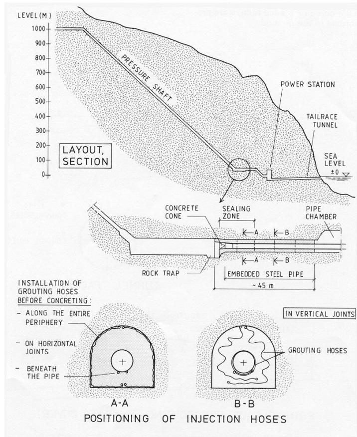
Fig. 17.4 Grouting of rock masses and concrete plug exposed to high water pressure
