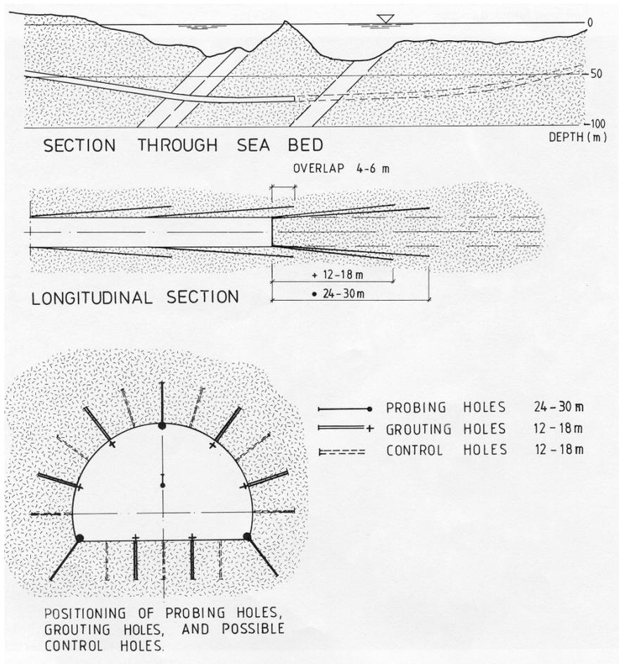
Fig. 17.1 Probing and pregrouting in sub sea tunnels
