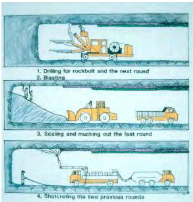
*Combined use of rock bolts and shotcrete. Shotcrete, and fibercrete, are used more and more in Norwegian underground works.
