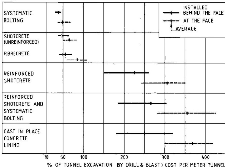
*Fig. III Important tunnelling items: Relative costs of rock support and tunnel excavation (drill & blast and mucking out)*
