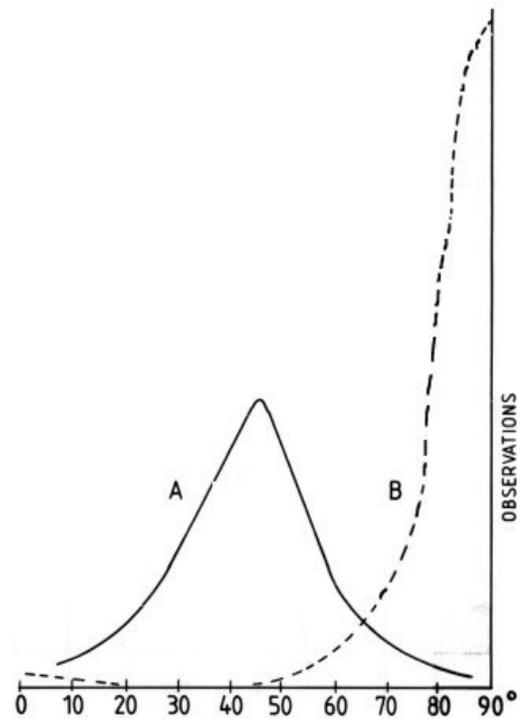
Fig. 7.6 Experience from 600 observations of water leakages connected to fractures. "A" shows the angle between the strike of the fracture and the adjacent regional fault. "B" the dip of the fracture.
