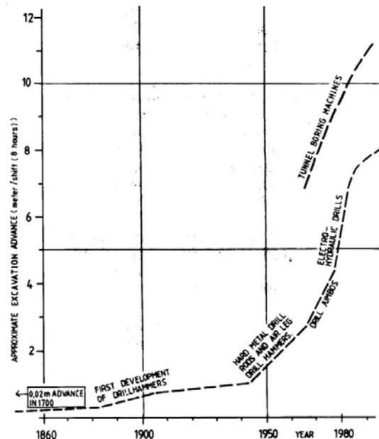
Fig. 1.1 Development of tunnel excavation
