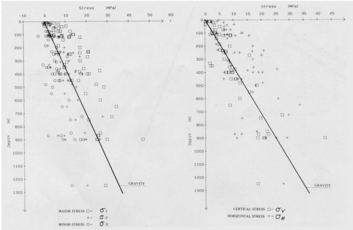
Fig. 5.1 Measured in situ principal stresses
