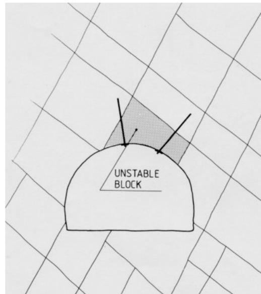
Fig. 8.4 Examples of local rock bolt support.
