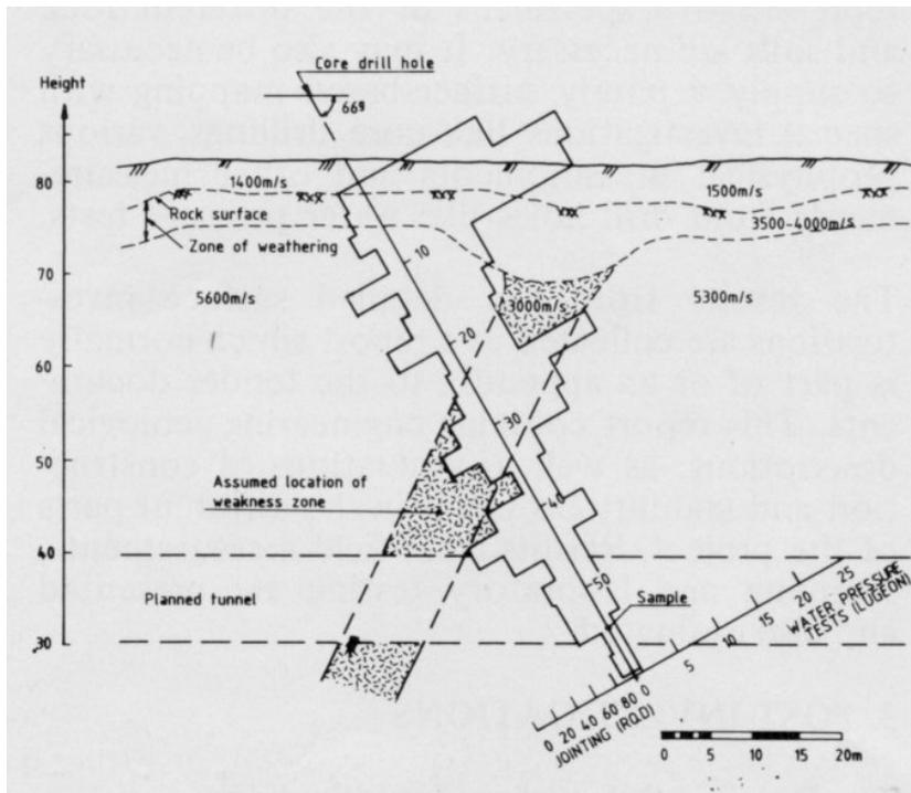
Fig. 6.2 Presentation of results from core drilling and seismic refraction measurements.
