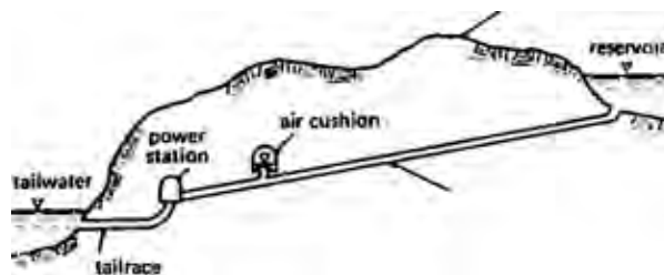
Fig. 1 Concept of powerplant with air cushion surge chamber.
