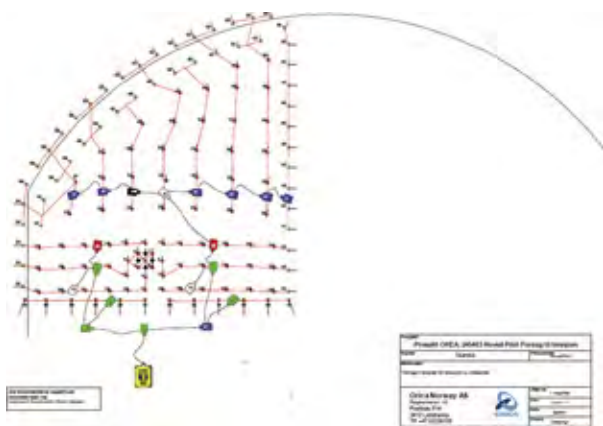
Figure 15. Drill pattern and charging plan for the pilot tunnel of the top heading in the main rock cavern.
