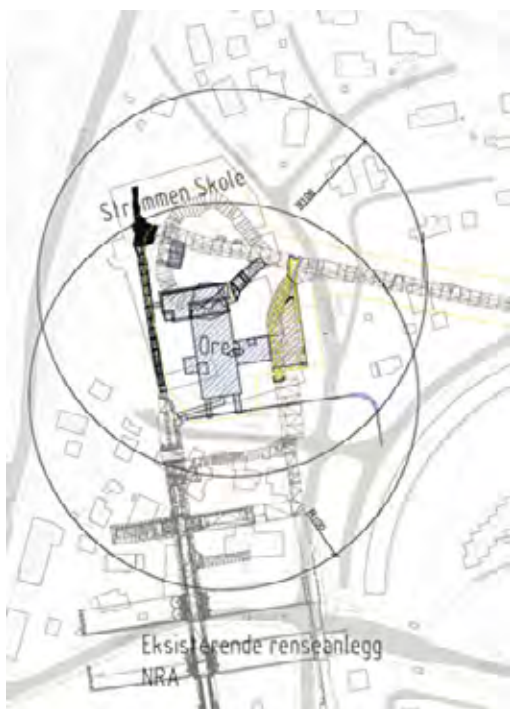
Figure 4. Assessment of area influenced by vibrations from blasting.
