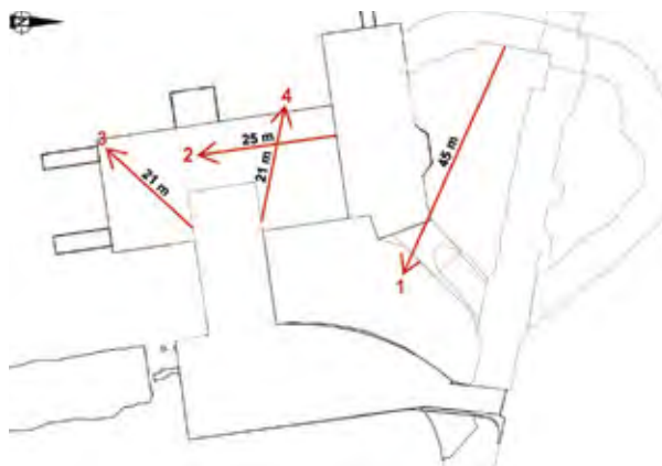
Figure 13. An overview of the drilled boreholes where the hydraulic jacking tests are conducted.
