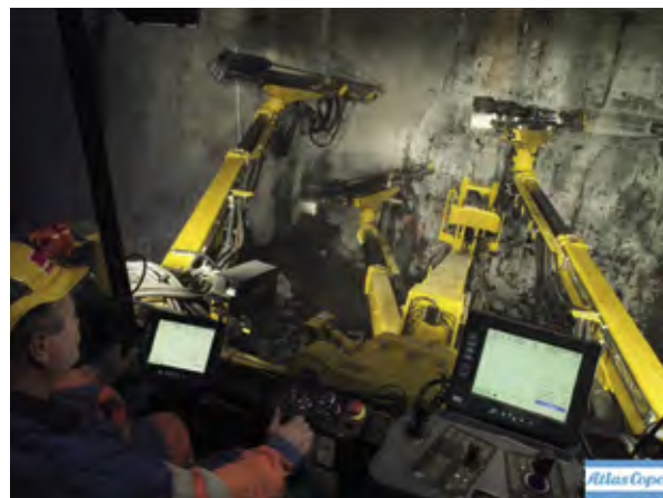
Picture 2 Drilling rig with 3 drilling booms and one basket. Atlas Copco (www.atlascopco.com)
