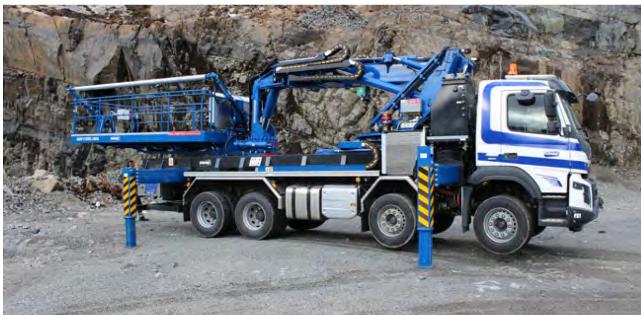
AMV QR Working Platform with interchangeable platforms in order to change between various baskets and can therefore be used for scaling, charging, bolt installation, general tunnelling works, membrane installation and PE foam installation.
