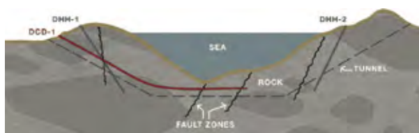
Figure 4: Directional borehole (red) turns horizontal and reaches fault zones in relevant area.
