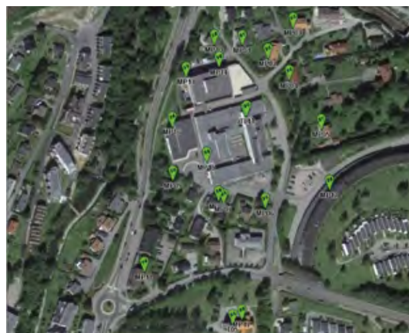
Figure 5. Location of instruments for measuring vibration in buildings during the construction stage.
