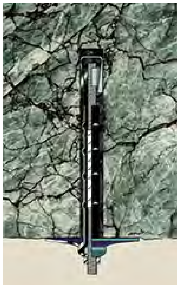
Image 14 - Installation of the CT-bolt by expansion shell
