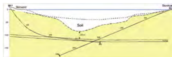
Fig. 5 Conventional and directional core drilling applied for investigation of critical part of the Oslofjord tunnel (based on Palmstrøm et al. 2003).
