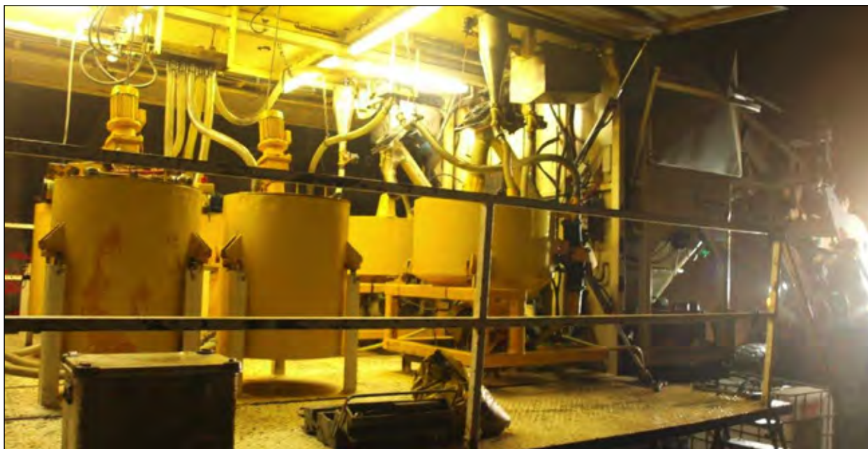
Figure 1: Filling of cement in big bags on a grouting rig
