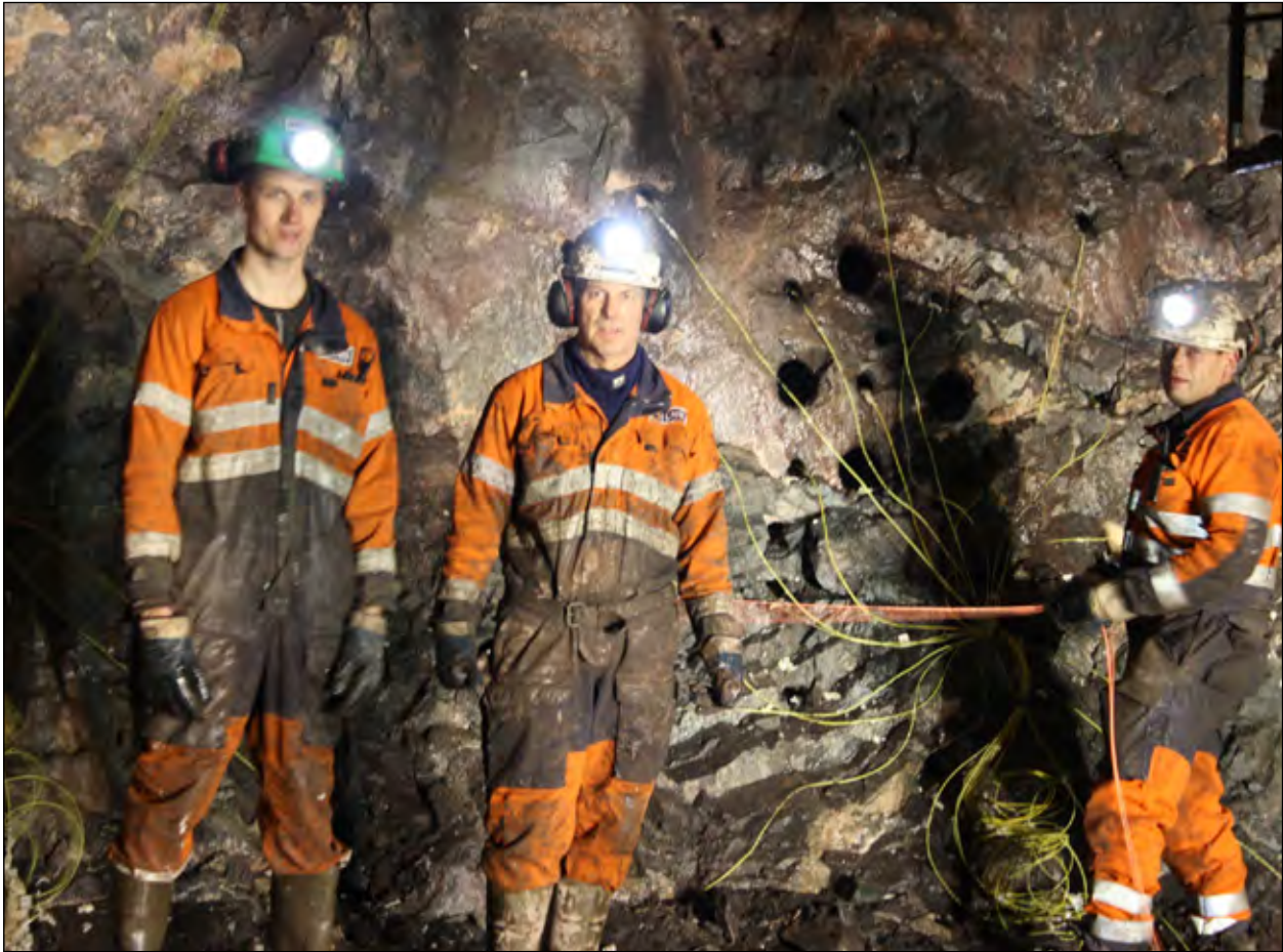
Crew at face charging the cut. Photo LNS
