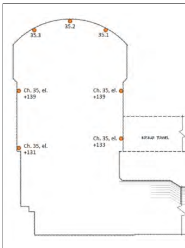
Figure 7. Convergence points installed in chainage 35, similar setup was used in chainage 17.
