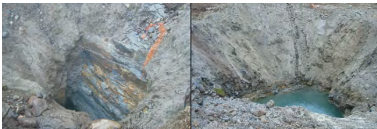
Fig. 2 - Sinkhole nearby Stutakvelven intake gate house in fully drained (a) and fully water filled (b) conditions (Courtesy: Norsk Hydro).
