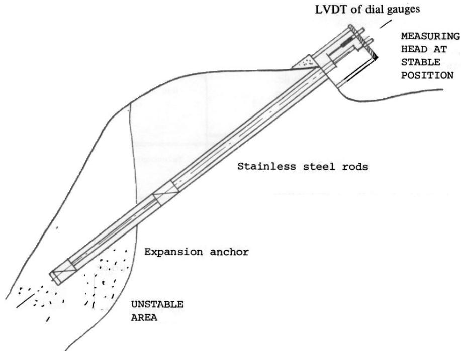
Fig. 4. Rod type multiple position borehole extensometer.
