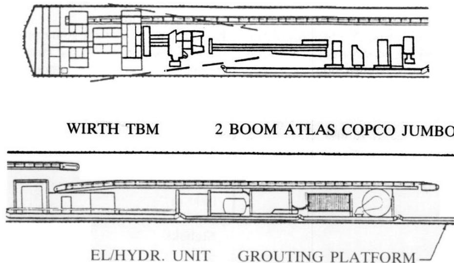
Fig. 2. TBM with grouting equipment incorporated.
