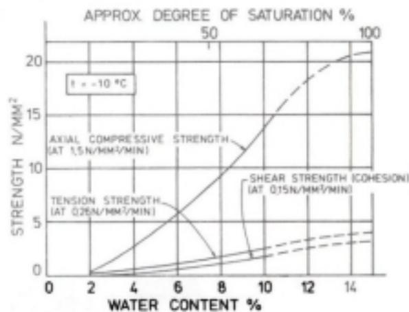
Fig. 5. Strength versus water content curves (Heiner's test).
