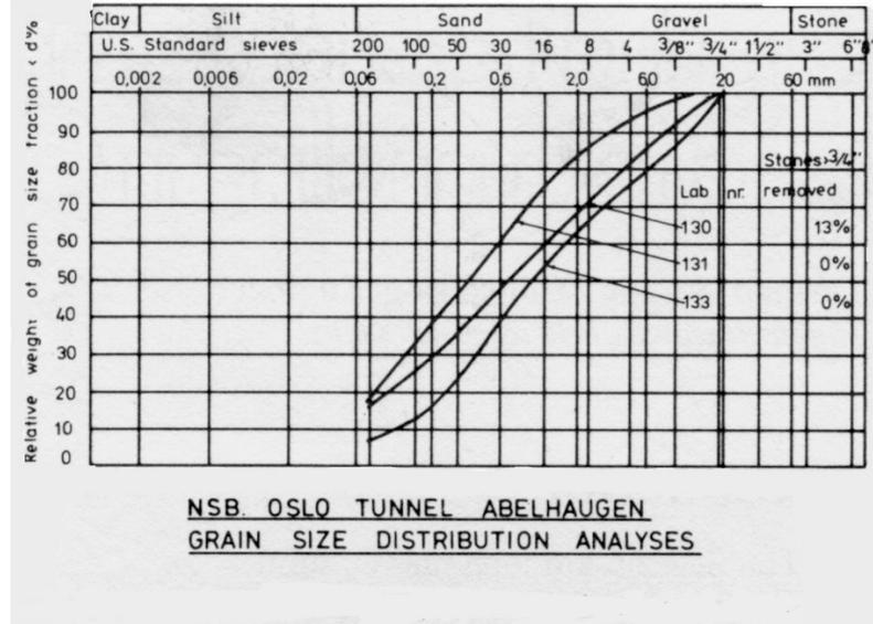
Fig. 3. NSB Oslo Tunnel Abelhaugen. Grain size distribution analyses.
