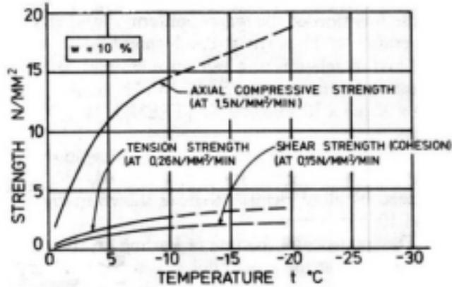
Fig. 6. Strength versus temperature curves (Heiner's test).
