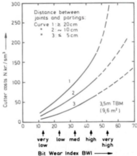
Fig. 2 Expected cutter cost for a 3,5 m TBM (with singel disc cutters) as a function of the Bit Wear Index and the intensity of weakness planes
