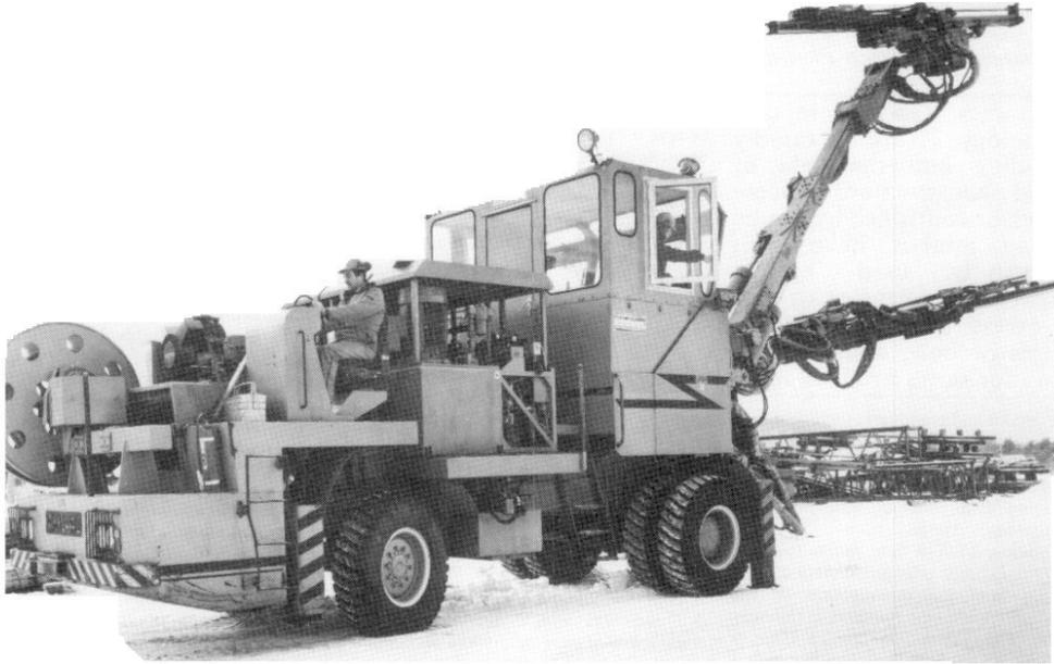
*Fig. 1. Computer controlled jumbo designed by Furuholmen.*
