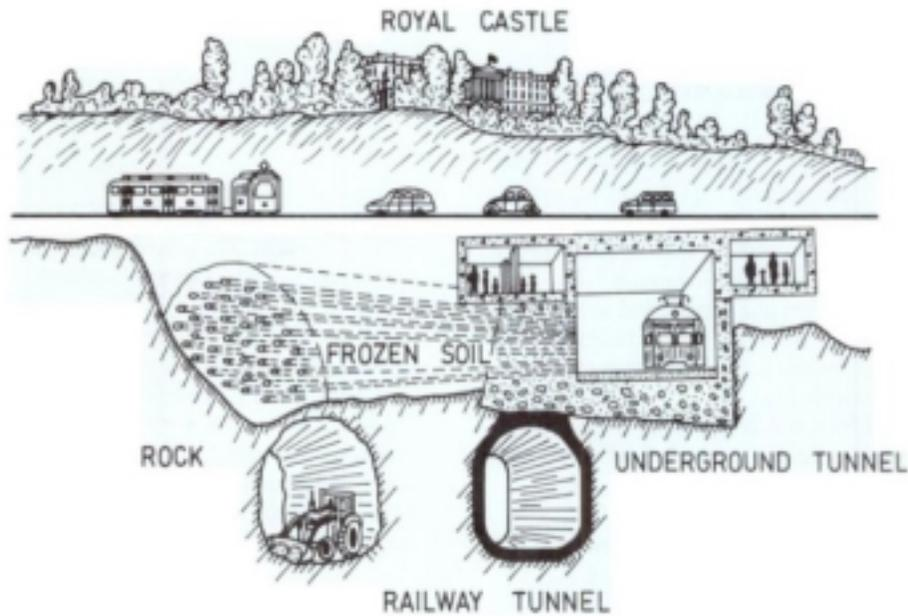
Fig. 4. Cross section of tunnel system.
