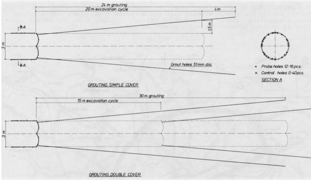
Fig 2. The principle of pregrouting.
