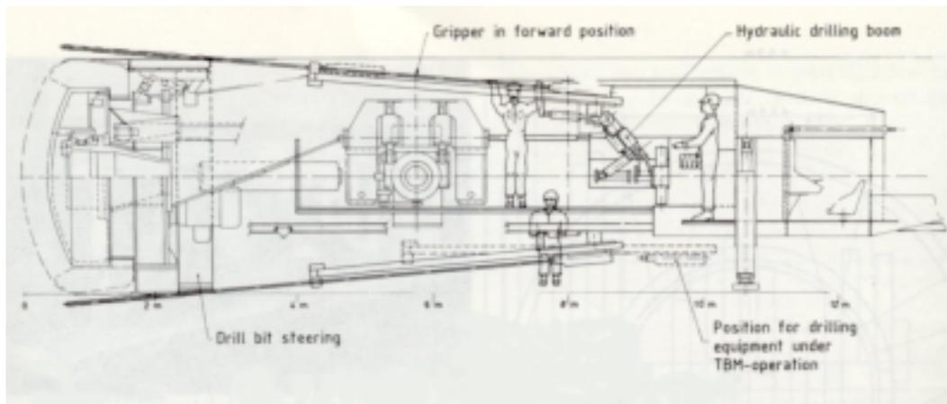
Fig 2. Mounting of drilling equipment on TBM.
