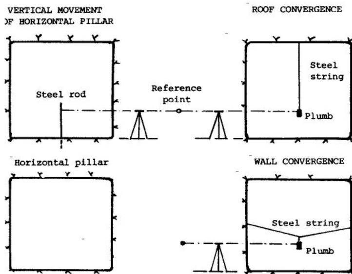
Fig. 2. Deformation measurements by levelling.
