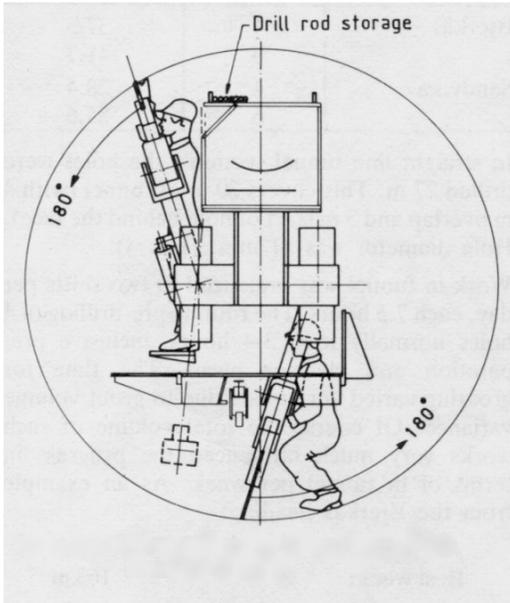
Fig. 3. Movement of booms carrying bore hammer.
