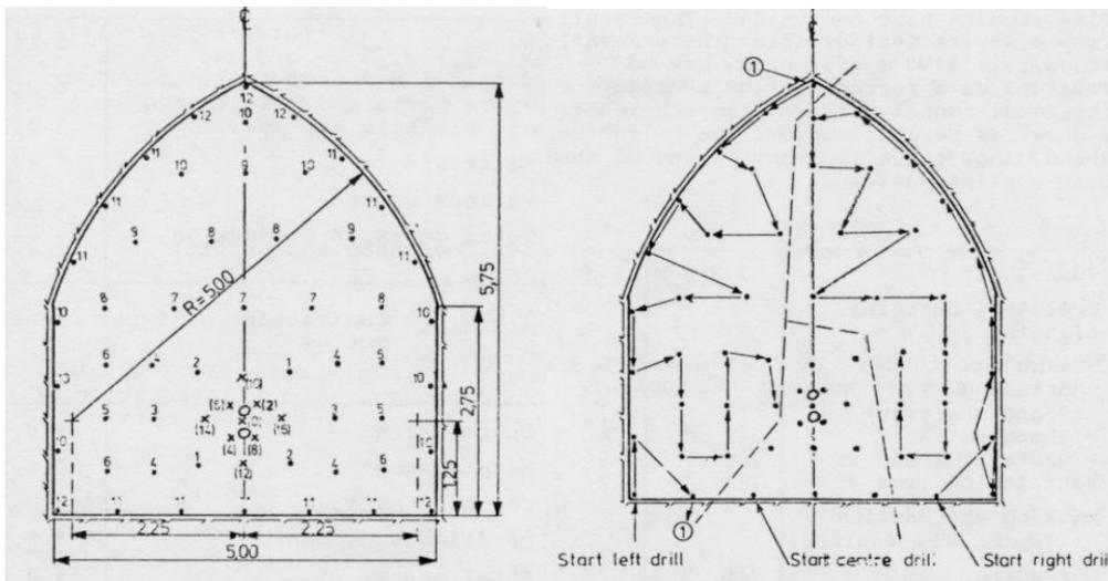
Fig. 3. Drilling pattern.
