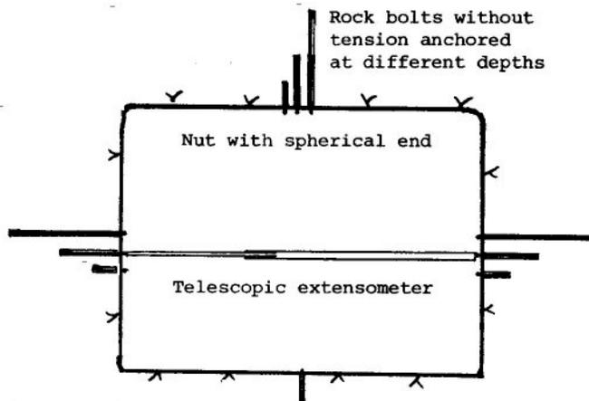
Fig. 3 Set up for rod extensometer measurements in a tunnel.
