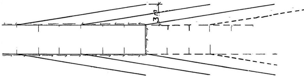
*Fig. 3. Drillholes for Pregrouting. Drill and Blast Tunnels.*
