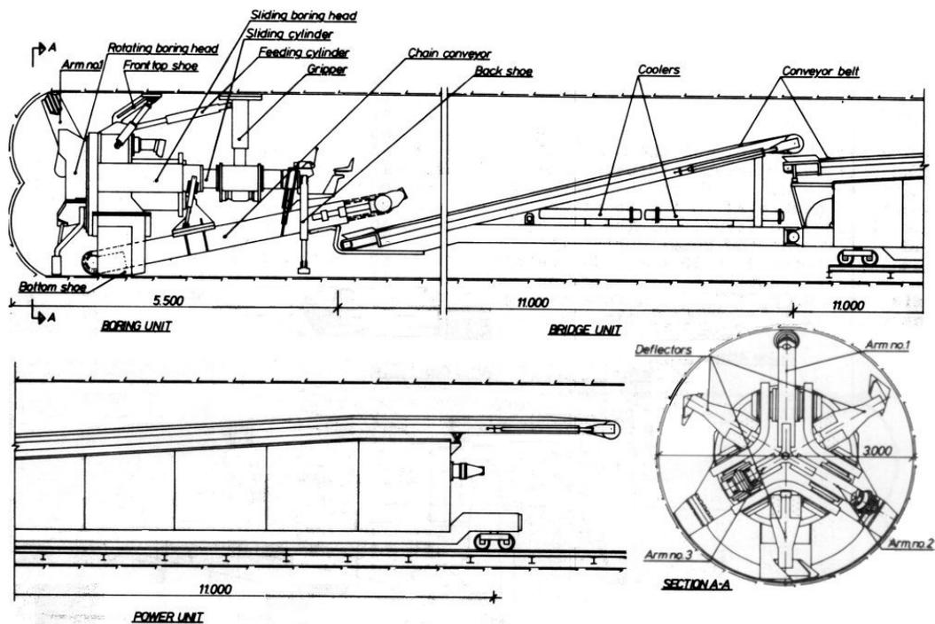
Fig. 3. The Bouygues Tunnel Boring machine.
