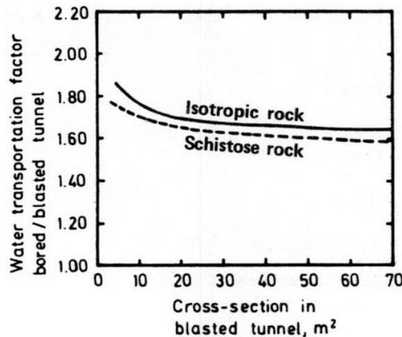
Fig 4. Relative water-transportation capacity of bored tunnels compared to blasted as a function of tunnel size.
