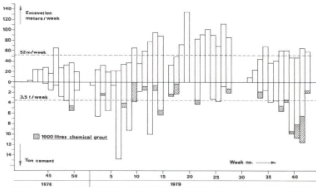
Fig 8 (top) Tunnel Holmen-Sandvika Progress-pregrouting
