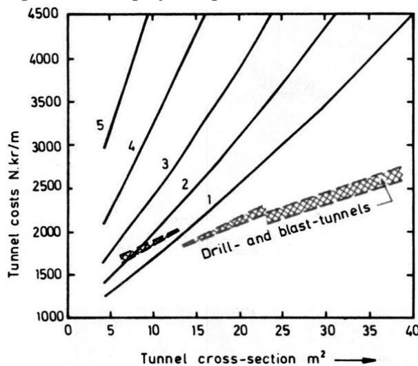
Fig.3. Unit cost for machine bored and conventional tunnels. Tunnel length 3 km.
