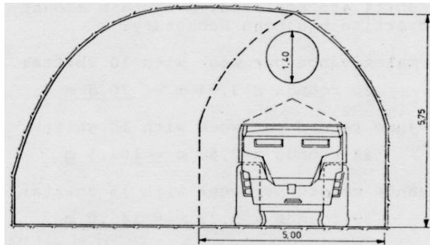
Fig. 6. Section, loading recess.
