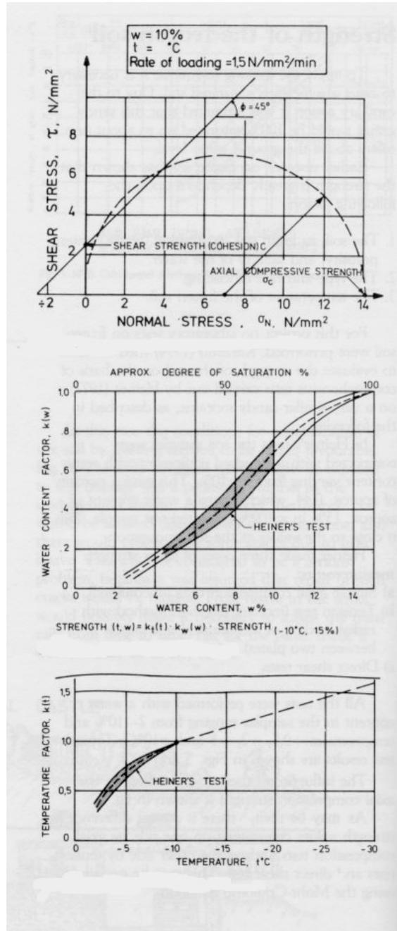
By calculating the bearing capacity of the frozen soil, a safety factor of at least 3 was applied in the actual design.
