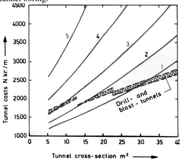
Fig. 5. Costs for machine bored tunnels (curve 1 to 5) compared with equivalent water-transporting capacity. Curve explanation as in figure 3.
