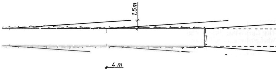
*Fig. 4. Drillholes for Pregrouting. TBM Tunnels.*
