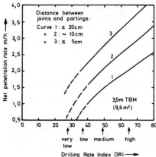
Fig 1. Expected net penetration rate for a 3,5 m TBM as a function of the Drilling Rate Index and the intensity of weakness planes in the rock mass.
