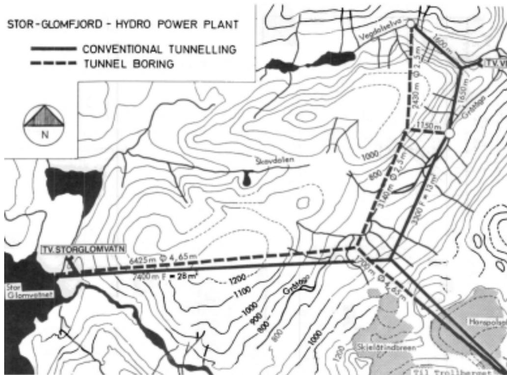
Fig. 6. Stor-Glomfjord hydro power project. With tunnel boring one adit including road building can be saved (in the north-eastern part of the project).
