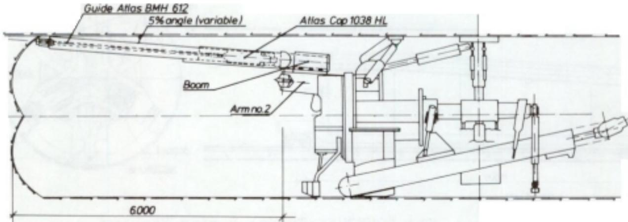
*Fig 4. Grout Hole Drilling.*
