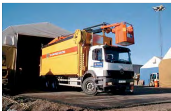
Figure 10. Andersen Mek. Verksted high pressure grouting rig.
