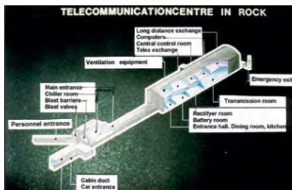
Fig. 3 Typical telecommunication centre in rock Welding the reinforcement steel bars in the concrete to a "Faraday Cage" solved protection against EMP.
