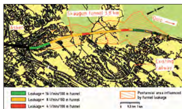
Figure 1: Areas of possible groundwater drawdown corresponding to the suggested leakage rates
