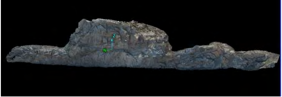
Fig 9 A. 3D model (complex 3D surface produced in PointStudio from dense point cloud) of slope profile 2450-2550L.
