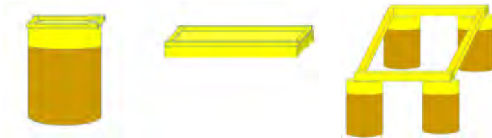
Figure 3 – Illustration of different foundation concepts; (a) Single suction caisson foundation & (b) Mud-mat foundation and (c) 4-can foundation
