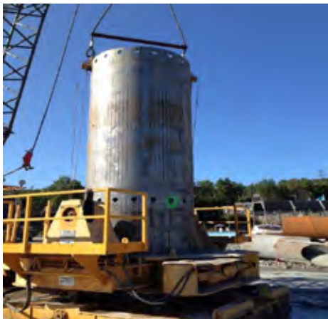
Figur 12: VRM 2500 Casing Oscillator
