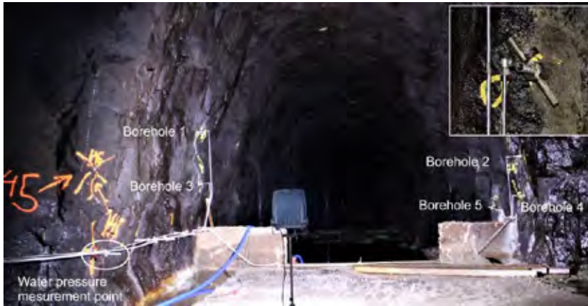
Figure 4. Location of boreholes in the tunnel looking upstream and a detail (top right corner).
