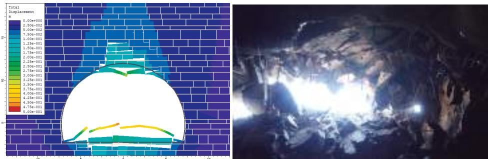
**Figure 7:** Example of a stability analyses for a tunnel in a jointed rock mass.
