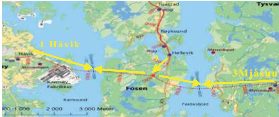
Figur 18-5 Driveretning for tunnel
