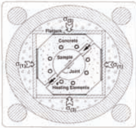
Figure 8. The CSFT apparatus used for MHT coupled-process joint tests in NGI's nuclear waste related projects for the Stripa SCV/SKB, Sellafield/UK Nirex Ltd, and URL/AECL studies. Makurat et al. 1990.
