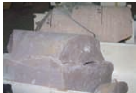
Figure 17. Two contrasting joints with JRC o values of about 1 and 16 according to back-analysed direct shear tests.
