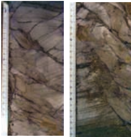
Figure 4. Core photo of heterogeneous and naturally fractured Middle Paleocene shale.
