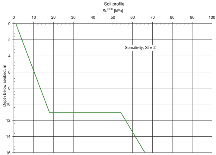
Figure 6 Illustrating a possible soil profile as basis for DIGIN results in Figure 7.
