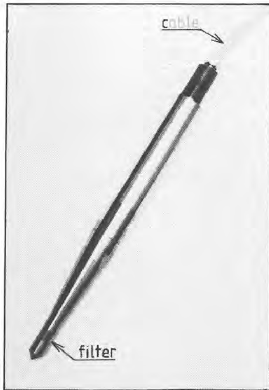
Fig. 34-1. The BAT pore pressure probe.
