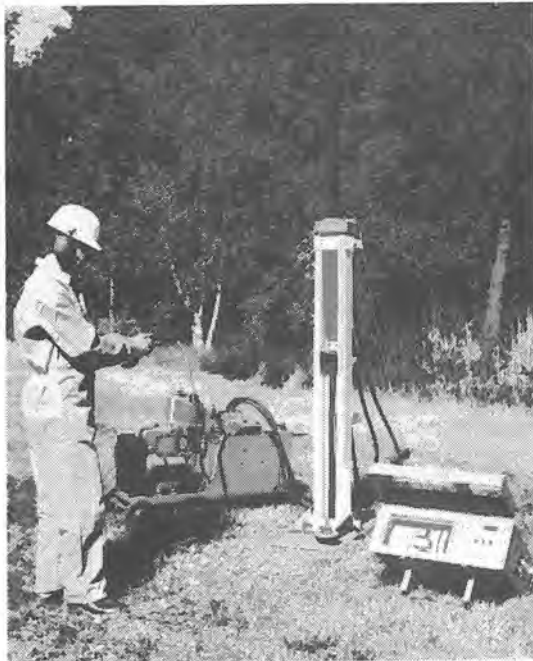
Fig. 34-4. The BAT pore pressure sounding equipment consists of an automatic registration unit, a pushing unit and a hydraulic power unit.
