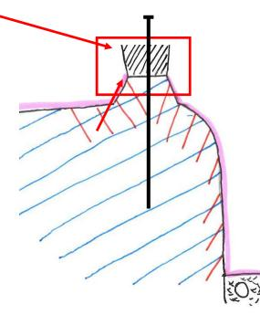
Red lines shows 12 mm, 70 cm lengths iron bars mounted in a cross pattern 25 x 25 cm To strenghten the alum shale body
