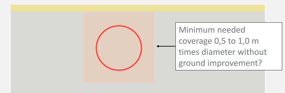
Tunneling with EPB or SS shields may be possible if the transition zones clay/rock are treated with jetgrouting
