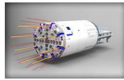
TBM to be equipped to perform probe drilling and pre-grouting
