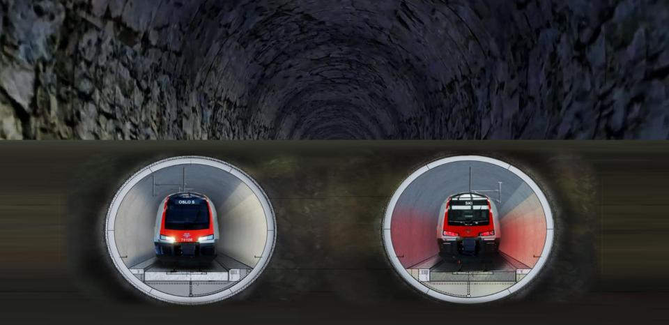
The tunnel is built with two separate tubes. Distance between the tubes is approximately 25 meters – CPs every 500 meters
