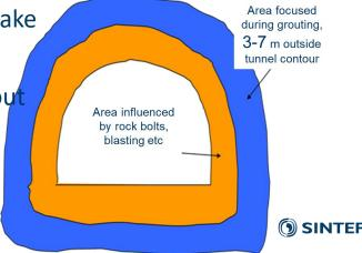
In principle; no matter excavation method the same concept of water control applies 'Rock mass grouting is 'first line of defence'
