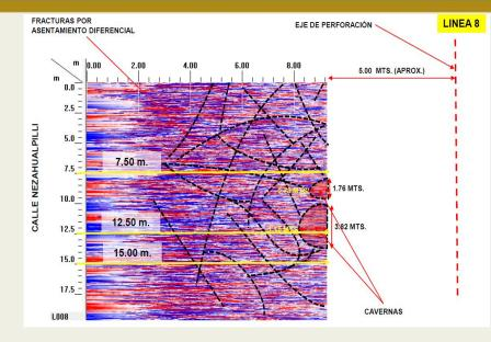
Underground Caverns (as detected by Georadar) Report Disclaimer: "THE RESULTS OBTAINED WITH THE USED SETTINGS INDICATE THE PHYSICAL CHARACTERISTICS OF THE STUDY AREA, ...HOWEVER IT IS NECESSARY TO TAKE INTO ACCOUNT THAT SOME STRUCTURES CANNOT BE CLEARLY DEFINED..."
