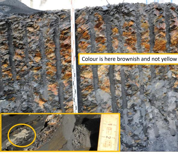
Galgeberg unit  $(3b\beta)$  in the Tøyen formation (3b). This black shale does not exhibit the same degree of lamination and fissile characteristics as in the alum shale (level 2). At Galgeberg the sufide grains/aggregates are encapsulated in baryte. The surface area accessible between sulfides and oxygen/moisture is consequently much lesser. Lower AP/NP potential Mechanical characteristics differs form alum shale. Joint characteristics are also different and clay mineral/mica content is lower
