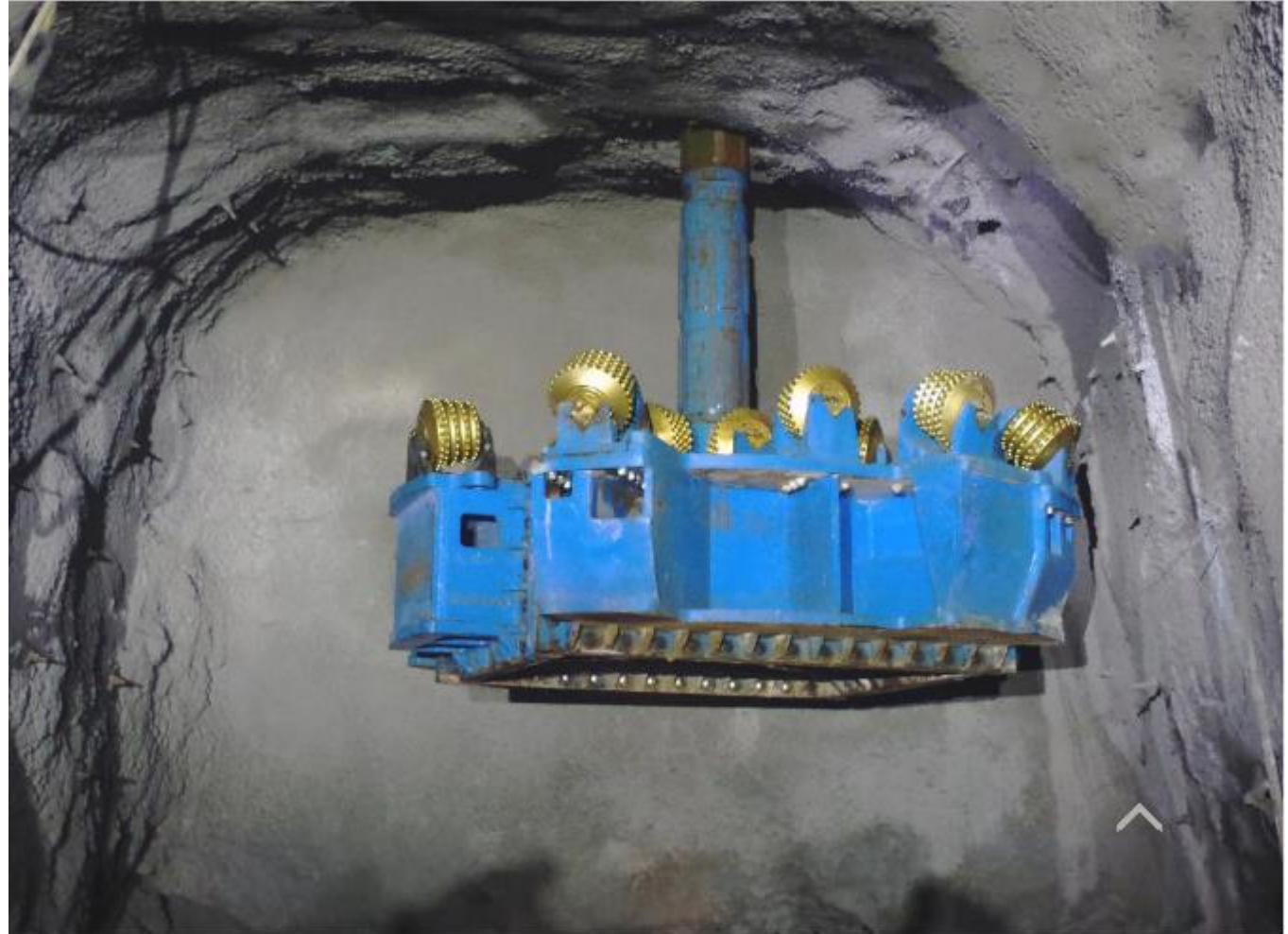
Raise boring. Foto: http://www.dmcmining.com
