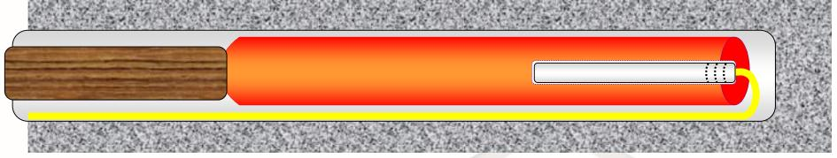
**Insert Detonator to its full depth**
