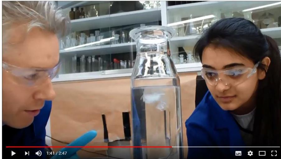
Microplastic fibers sink with turbulence - a lab demonstration
