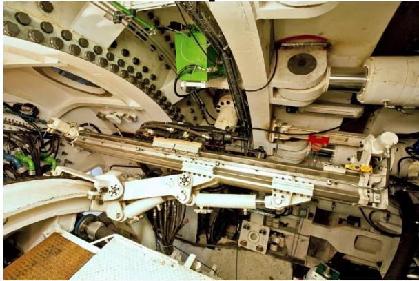
Two permanent installed front drills for face drill pattern
