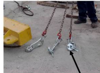
Blow up lifting lug and ring clutch
