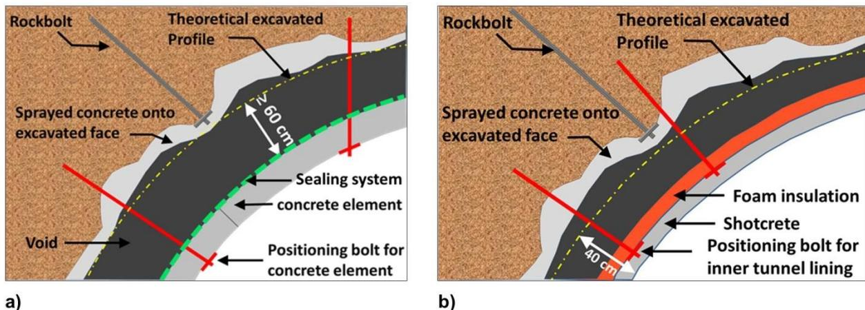
**Figure 1. (a) Inner lining with precast concrete elements; (b) foam isolation – sprayed concrete lining (after [4]).**
