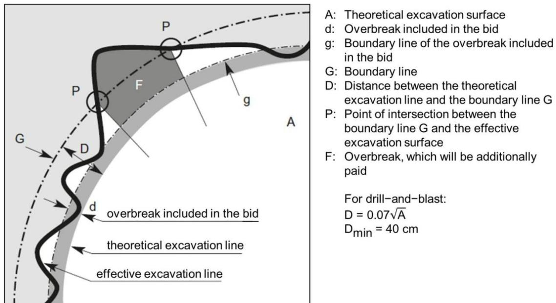
Figure 4. Overbreak regulations for drill-and-blast excavation according to the Swiss standards [8].
