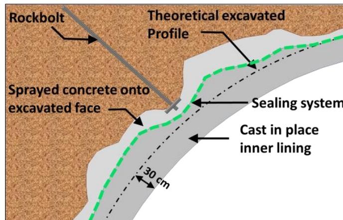
**Figure 2. Inner lining with cast-in-place concrete (double-shell lining).**
