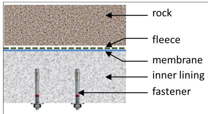
**Figure 8: Fixing of installations with dowels.**
