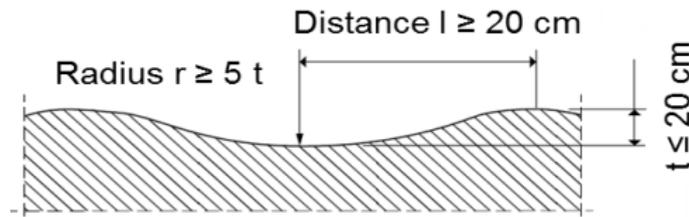
**Figure 6. Acceptable unevenness for the sealing membrane [10].**
