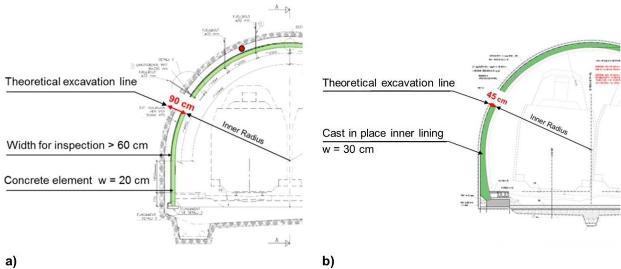
**Figure 3. Theoretical excavation line for, (a), inner lining made of precast concrete elements (after [6]) and, (b), inner lining made of cast-in-situ concrete (after [7]).**
